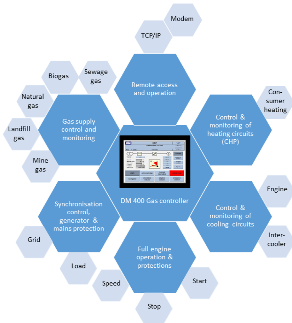
Fig. 1: DEIF Fully integrated gas engine and CHP control system
