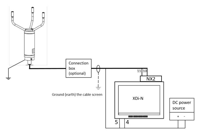
**NOTE** The stainless steel mounting base on the WSS 750 <u>must</u> be connected to the ship's metal hull or another good ground connection.
