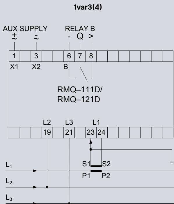
Shown contact positions: Aux. voltage not connected
