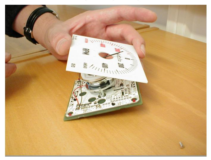
This is the most critical part of the operation. Be very careful not to bend or stress the pointer or instrument system. This could damage the system or cause increased inaccuracies.
