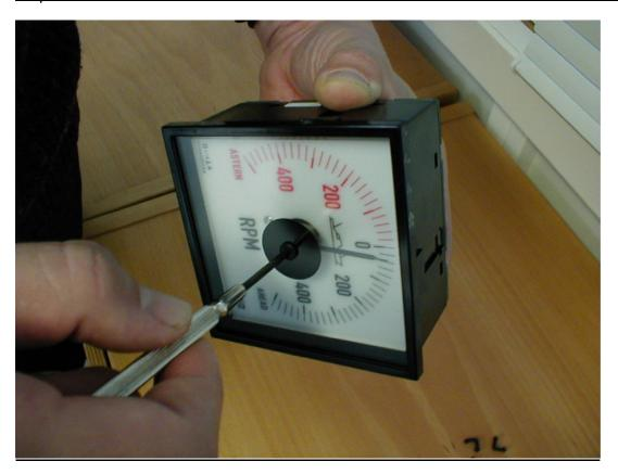
Step 7. Mount the clips again and then make a zero adjustment.
