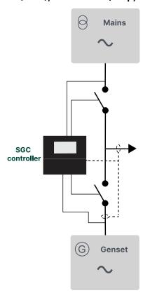
**AMF:** If there is a significant loss of mains power or a total blackout, the controller automatically changes the supply to the generator. This makes sure that there is power during a mains failure and prevents damage to electrical equipment.
