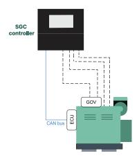
**Engine drive:** Use the controller to control one engine. The controller has all the necessary functions to control and protect the engine.
