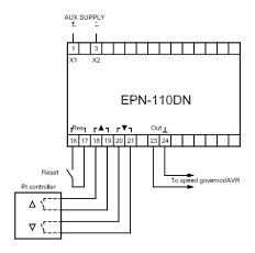
A 2A fuse may protect the auxiliary supply connection.
