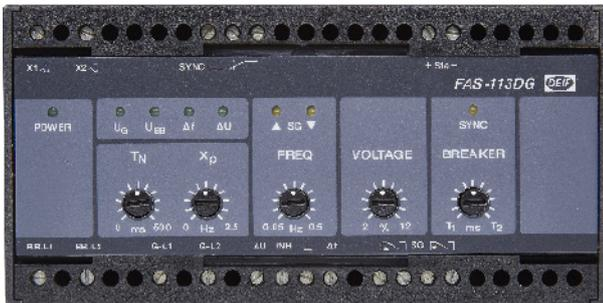
The FAS-113DG synchroniser is applied for synchronisation of a generator to the busbar and closing of its circuit breaker when the voltage difference, the slip frequency and the phase angles are within the preset limits.
