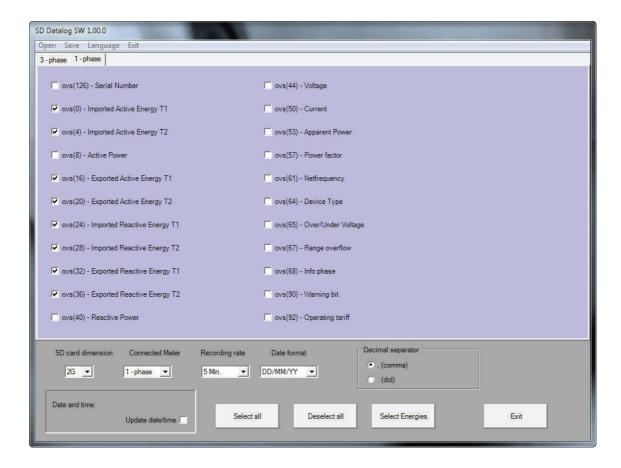
The "1-phase" section shows the list of available values when the device is connected to a single-phase meter.
