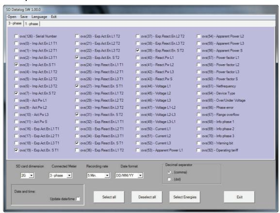
The "3 – phase" section shows the list of available values when the device is connected to a three-phase energy meter or a three-phase power meter.
