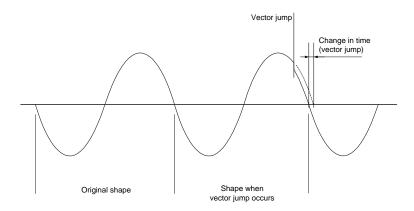
Again, comparing the sine curve time duration with the previous ones, a sudden change in time can be detected. This is the vector jump.
