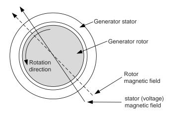
If a mains failure occurs, the time lag of the stator magnetic field (and the output voltage) will change (jump). This is called a vector jump.
