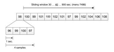
The numbers in the above figure represent the busbar voltage as a percentage of the nominal busbar voltage.
