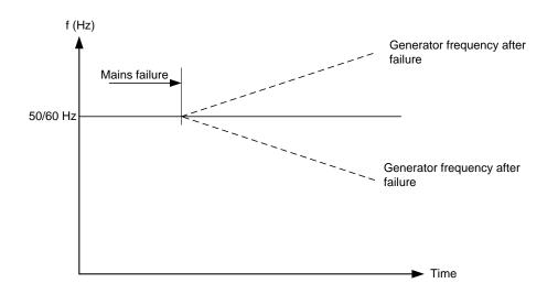
So, a dramatic drop/increase of frequency over time is a mains failure. The df/dt setting is made in Hz/sec.
