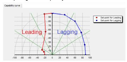
If the set point for reactive power is outside the limiting curve, the controller stops reactive power (or cos phi) regulation. When the reactive power set point moves inside the limiting curve, the controller regulates reactive power (or cos phi).
