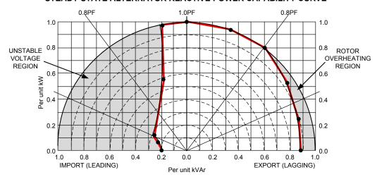
The settings of points 1-6, leading and lagging, should represent the generator manufacturer's recommended settings for var import (-Q)/export (+Q). Notice that the above curve is just an example, the actual values must be obtained from the generator manufacturer.
