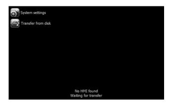
In this case, the Runtime will be automatically installed into the panel from AGI Creator at the first project download.
