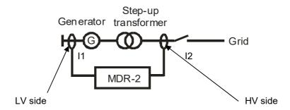
Due to the step-up transformer, the CTs have different ratios. This is handled by two different settings for the LV (generator) side and the HV (consumer/grid) side CTs.
