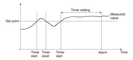
The output is activated when the timer runs out. The total delay will be the delay setting + the reaction time.
