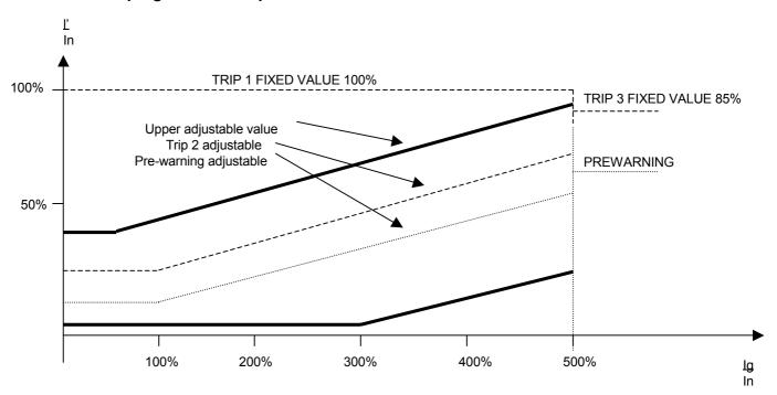
The trip curve shows that if the generator current (Ig) exceeds the nominal value (In) MDR-1 will start compensating for the differential current (I') simply by moving the trip and warning setpoint values upwards as the generator current increases. This will compensate for the previously mentioned measuring imbalances.
