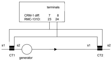
The differential current (measured on the terminals) occurs as a result of the connection between CT1 and CT2.
