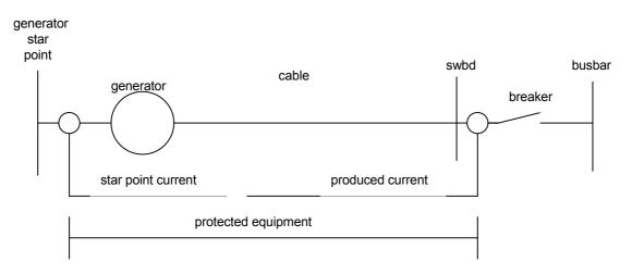
The differential current is the difference between the current measured in a phase in the generator terminal box (star point) and the current measured in the same phase in the switchboard. This value should be zero but due to imbalance in the measuring circuits (current transformer deviations, measuring input deviations etc.) a deviation occurs.
