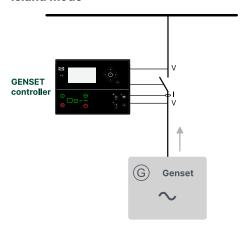
Island mode operation is typically used in power plants that are isolated from the national (or local) electricity distribution network. There are two key types of island mode operation:
