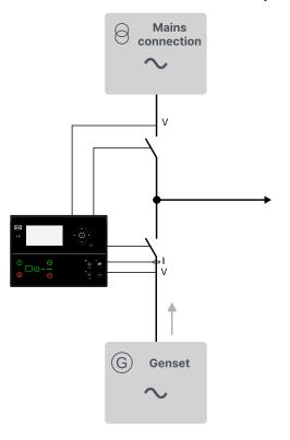
**Automatic Mains Failure (AMF):** If there is a significant loss of mains power or a total blackout, the controller automatically changes the supply to the emergency generator. This makes sure that there is power during a mains failure and prevents damage to electrical equipment.
