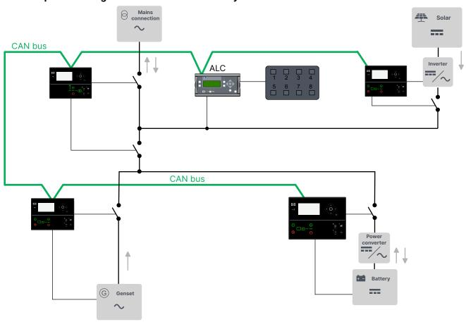
**NOTE** The iE 150 Genset Hybrid controller cannot be used in a power management application.
