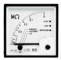
The SIM-Q supervises the insulation resistance between an insulated voltage distribution network and an earth/safety cable. The advanced measuring sequence performs an automatic offset adjustment to eliminate possible effects of uneven stray capacitance and DC voltages.
