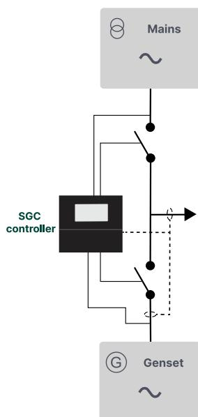
**AMF:** If there is a significant loss of mains power or a total blackout, the controller automatically changes the supply to the generator.
