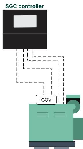
**Engine drive:** Use the controller to control one engine. The controller has all the necessary functions to control and protect the engine.
