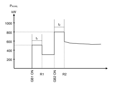
To connect the load groups individual relays can be selected on each AGC or on one of the AGCs only. This depends on the number of load groups that need to be connected and also on whether the function has been given ON or RUN status.
