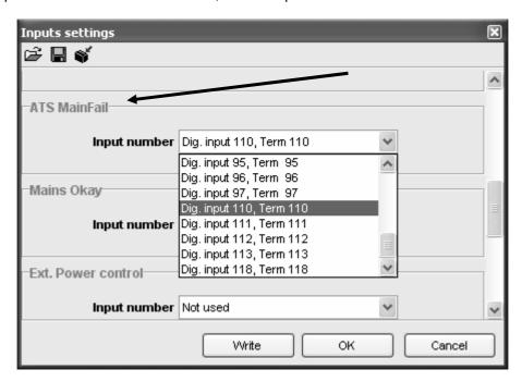
The mains unit will not try to operate the ATS (mains breaker) at all. But it is still necessary that position feedbacks are wired up.
