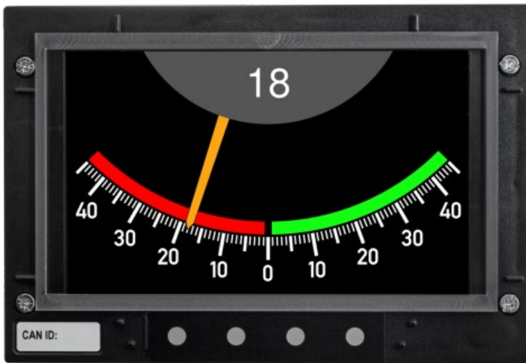
Fig. 4.1 XDi 144 D or M when the front frame is removed – the 4 pushbuttons are available
