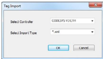
CODESYS V3 Development System generates a new version of the \*.xml file each time the PLC project is built.
