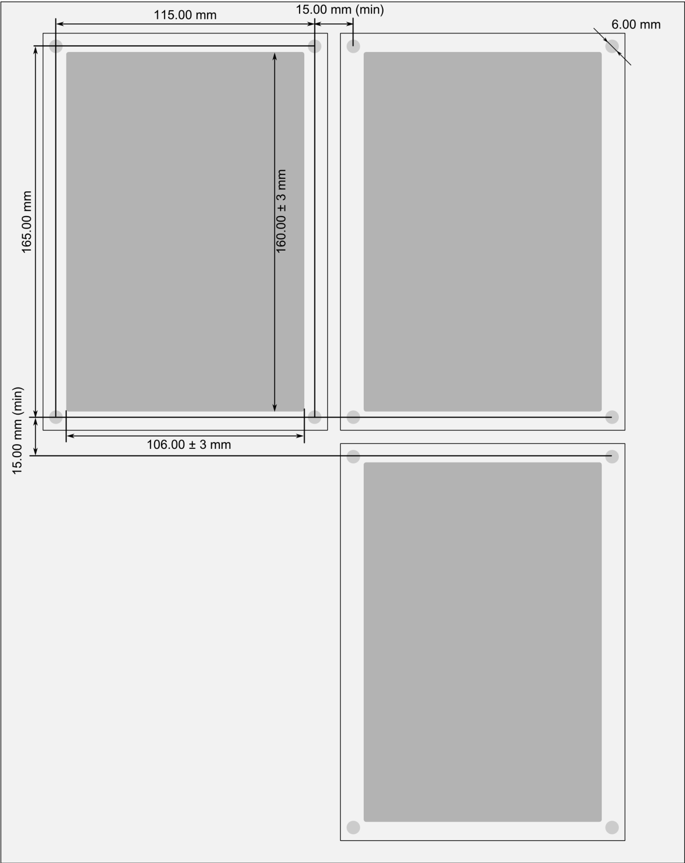
Figure 2.3 Panel cut-out and spacing of the IED.
