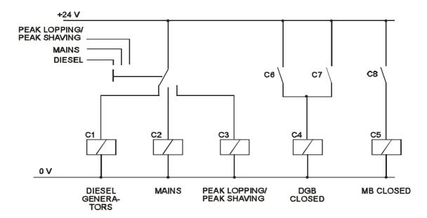
The selector switch is the operator's selector for diesel generator running or mains connection. Note that for the switching to take effect, the GPCs must be in "remote" mode (selected on the display).
