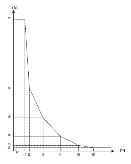
The inverse time characteristic for the overcurrent protection is illustrated above – the t's and i's refer to the six set points giving the slopes of the curve. Notice that the curve is extended horizontal from (i6, t6) to ( $\infty$ , t6) indicating that a current higher than i6 corresponds to a delay equal to t6.
