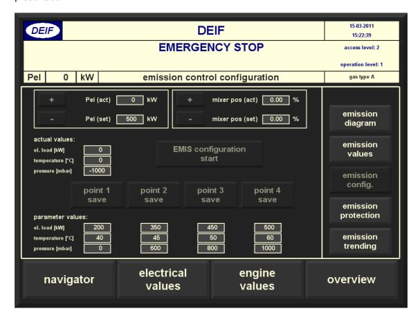
The generator must be parallel with mains when entering this page.
