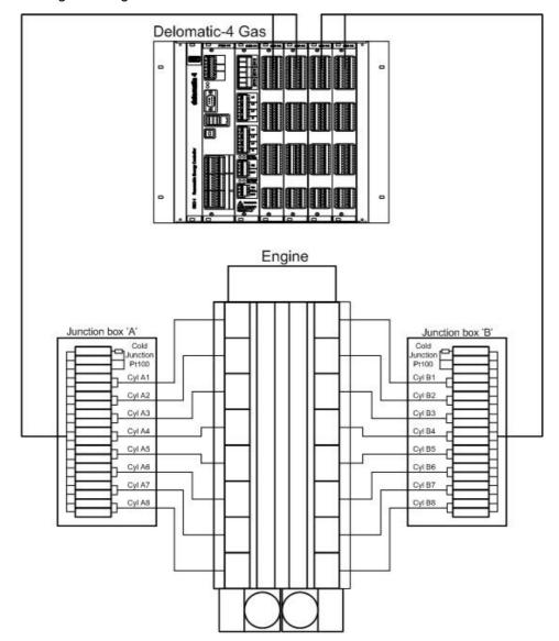
The above example shows a 16-cyl. engine. Engine sizes up to 20-cyl. are supported.
