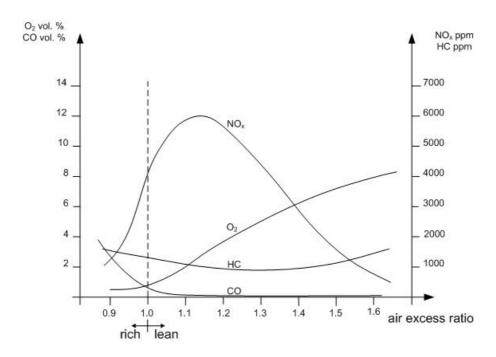
The curves show that the  $NO_x$  value decreases with an increasing excess air ratio, so in theory the mix should be as lean as possible. On the other hand, the HC content increases when the air excess ratio exceeds approx. 1.35, so the resulting air excess ratio will be a compromise. Finally, if the air excess ratio gets too high, the mix gets so lean that misfiring will take place.
