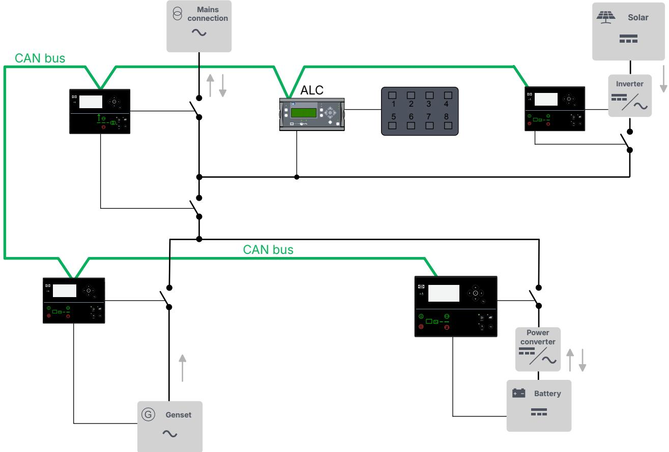
**NOTE** You can use AGC 150 generator, mains, and bus tie breaker controllers for power management in a hybrid system. However, the AGC 150 genset hybrid controller cannot be used in a power management application. To control the photovoltaic (PV) power source(s), use ASC 150 Solar.
