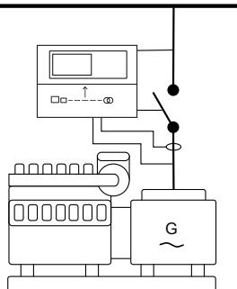
Island mode operation is typically used in power plants that are isolated from the national (or local) electricity distribution network. There are two key types of island mode operation:
