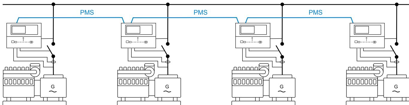
Power plant with synchronising generators. Can also be used in critical power plants with a start signal from an external (ATS) controller.
