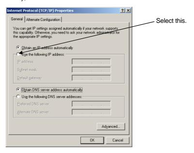
Write IP address = 192.168.2.22 (option N processor card IP address + 1), and Subnet mask = 255.255.255.0. Do not write any default gateway address. As regards the DNS server, it is not necessary to write anything, but if you know the DNS IP address, you can write it there (e.g.: 10.0.0.11).
