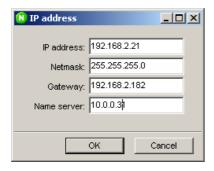
Press the 'OK' button for writing the new configuration to the multi-line 2 unit.
