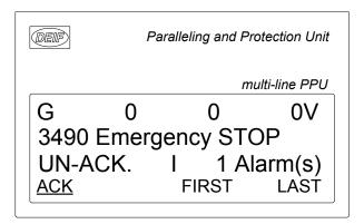
This display example indicates an unacknowledged alarm. The display can only show one alarm at a time. Therefore, all other alarms are hidden.
