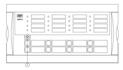
The AOP-2 has a separate push-button (1) for the combined lamp test and dimmer functionality. A short activation of the push-button will activate the lamp test function. If no further action is taken within three seconds, the AOP-2 will turn back to normal indication.
