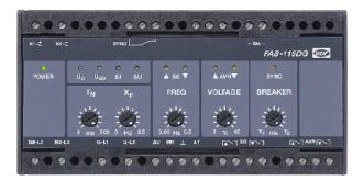
The FAS-115DG synchroniser is applied for synchronisation of a generator to the busbar and closing of its circuit breaker when the voltage difference, the slip frequency and the phase angles are within the preset limits. Moreover, this synchroniser offers voltage regulation.
