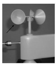
Replacement of the defective 3-cup rotor.
