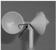
Remove the sealing wax in the bolt hole of the defective 3-cup rotor.
