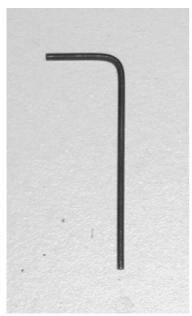
Necessary tool: 1,6 mm Allen key (1/16 inch)
