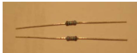
Two CAN resistors 120 Ohm
