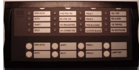
The AOP-2 (Additional Operator Panel)
