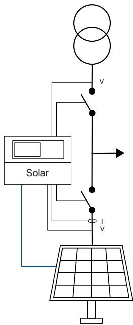
**Fixed power:** When given a signal, the controller starts, synchronises, and connects the PV. After the breaker closes, the controller ramps up the load to the set point level. When the stop command is given, the PV breaker is de-loaded, opened and the PV is stopped.
