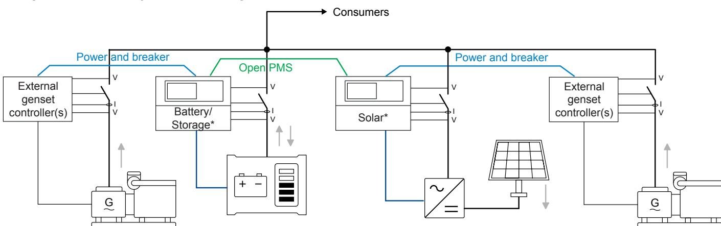
**NOTE** \* You can use multiple controllers in the application. Power measurements can be connected to the closest battery/storage or solar controller.
