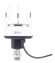
The ultrasonic measuring principle with no moving parts gives reliable performance without any wear-out problems and without requiring regular service.
