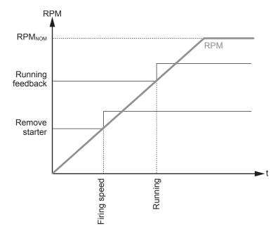
The diagram illustrates how the remove starter input is activated when the engine has reached its firing speed. At the running speed, the digital running feedback is activated.
