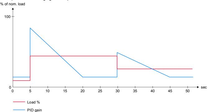
The diagram above shows the reaction of the gain, based on two load changes.
