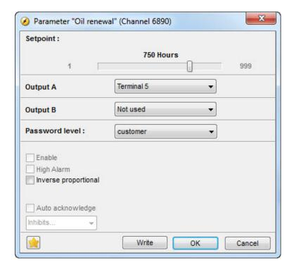
When the running hours counter has reached 1000 hours, the controller will reset the hours just for the oil renewal function. If, for example, the set point has been set to 750 hours and inverse is not enabled, the relay will close at 750 hours and remain closed until 1000 hours is reached, and then the hours counter starts from 0 hours again.
