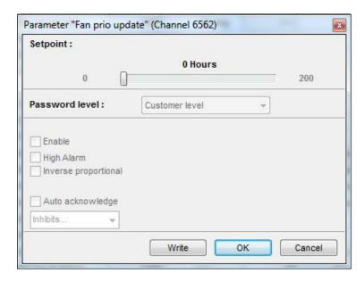
If the fan priority update is set to 0 hours, the order of priority will be fixed at: Fan A, fan B, fan C and fan D.
