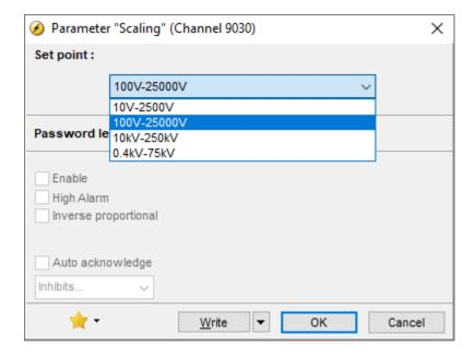
Changing the voltage scaling changes the ranges for voltage, power and transducer output parameters.
