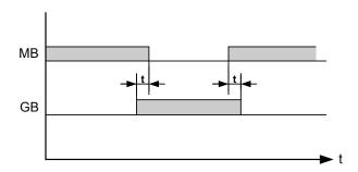
The diagram shows that when the generator breaker is synchronised, the mains breaker will be opened automatically after a time delay (t). Later the mains breaker is synchronised, and the generator breaker is opened after the time delay (t). The time delay is measured in seconds and can be adjusted from 0.10 to 99.90 seconds.
