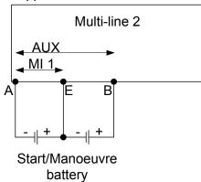
The power supply measurement is used as the reference RF1 (points A and B) in menu 6432 and multi-input 1 is used as the type T1 (points A and E) in menu 6431. By making these measurements, it is possible to calculate the voltage between E and B. This gives a full picture of battery voltages, for example:
