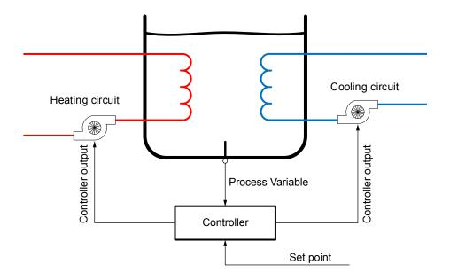
For this application, two controllers must be configured: one with direct output for the heating pump and one with inverse output for the cooling pump. To achieve the illustrated inverse output, an offset of 100 % is needed. See the sections about "Analogue offset" and "Example of inverse output with 100 % offset" for more information regarding offset.
