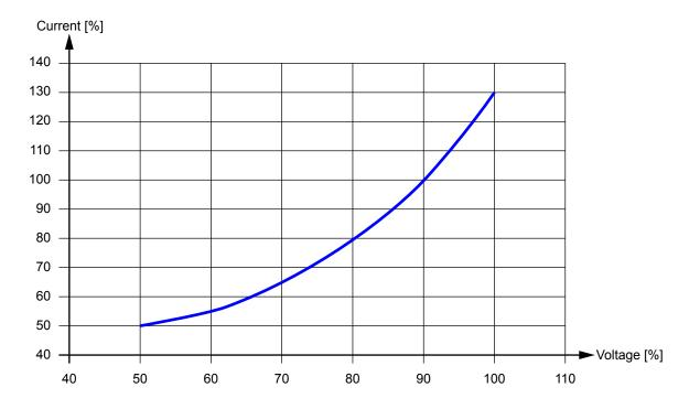
When the actual values represent a point above the curve, the breaker should be tripped. The curve shows that the generator breaker will trip when two requirements are met: The generator voltage is below 50 % of rated, and the current is above 50 % of rated.
