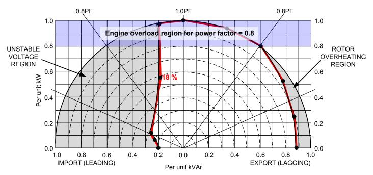
The alternator 100 % load is the outer circle, and the engine 100 % load is the bottom of the blue block. With the operating chart it is possible to see where the alternator-safe line is closest to the 1.0 PF line. In this operating chart each vertical line represents 10 %, and so the point closest to 1.0 PF is 18 %. Use the nominal alternator values and the nominal engine values to do the calculations.
