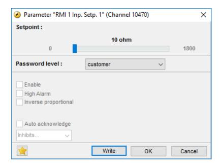
Adjust the resistance of the RMI sensor at the specific measuring value. In the example above, the adjustment is 10  $\Omega$  at 0.0 bar.
