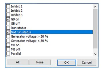
In this example, inhibit is set to *Not run status* and *GB ON*. Here, the alarm will be active when the generator has started. When the generator has been synchronised to the busbar, the alarm will be disabled again.
