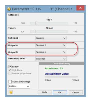
The timer configured in the alarm window is an ON delay that determines the time during which the alarm conditions must be met before activation of any alarms or outputs.
