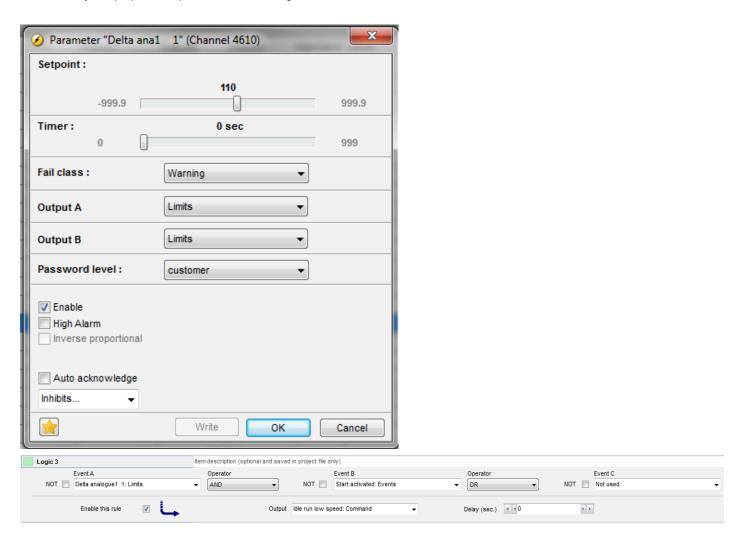
In order for this function to work, menu 6295 Idle active must be enabled, and the relay output must be configured. Otherwise the low speed function will not work.
