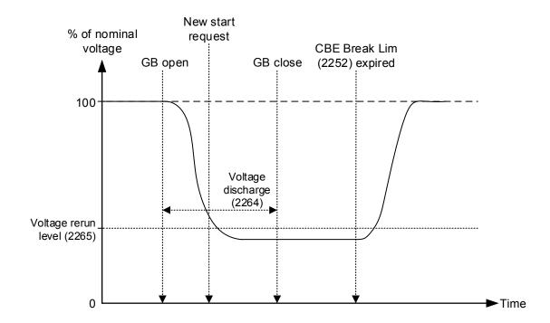
In the diagram above, the excitation is shut off as soon as the breaker is opened. Shortly after the breaker is opened, a new start request appears. The controller will wait with the closing of the GB until the "voltage discharge timer" has expired.
