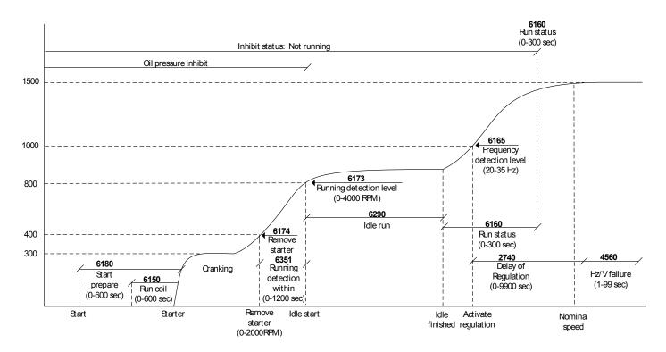
The set points and failures in this overview are the same as described in the chapter "Start-up overview", except for the idle run function. This function is described in the chapter "Idle running".
