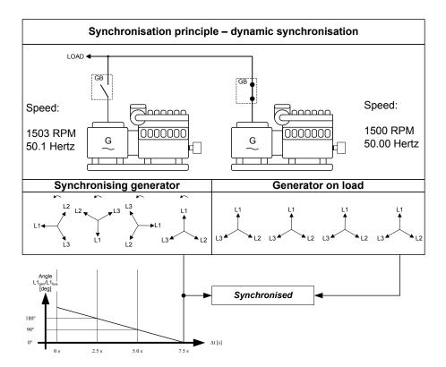
In the example above, the synchronising genset is running at 1503 RPM  $\sim$  50.1 Hz. The generator on load is running at 1500 RPM  $\sim$  50.0 Hz. This gives the synchronising genset a positive slip frequency of 0.1 Hz.
