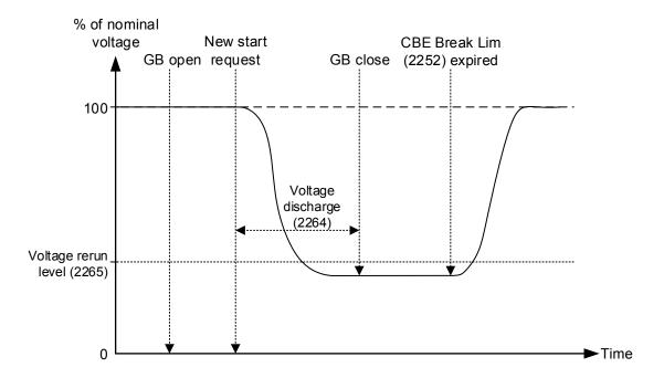
In the diagram above, the excitation is ON during cooldown. Then a new start request is made, which means that the excitation will be shut off. When the excitation is shut off, the voltage discharge timer starts.
