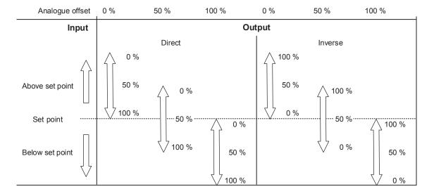
100 % offset is commonly used with inverse output, like in the previous cooling example. For an example of other use, see "Example of inverse output with 0 % offset".
