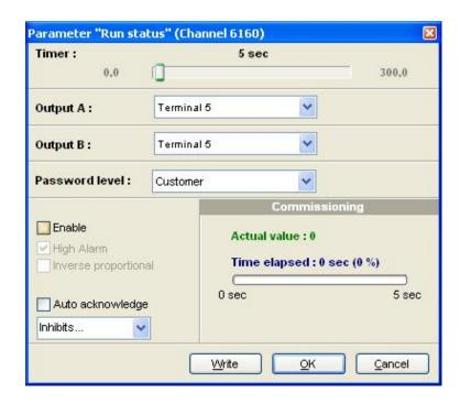
Select the correct relay number in output A and output B and enable the function. Change the relay function to limit in the I/O menu. Then the relay will activate, but no alarm will appear. Note that to avoid an alarm, both output A and output B need to be configured to a relay.
