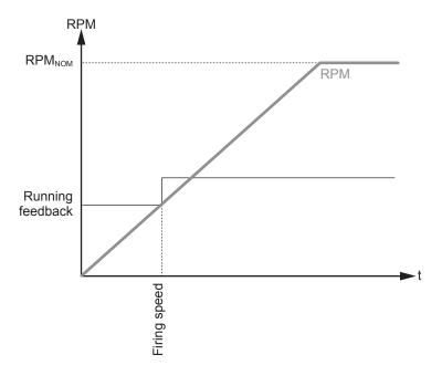
The diagram illustrates how the digital running feedback (terminal 117) is activated when the engine has reached its firing speed.
