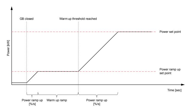
The warm up ramp activation is enabled and the input is configured via *Warm up type* (parameter 2961). The activation of the warm up ramp input limits the available power of the genset to the percentage level configured in *Power ramp up* (parameter 2612).
