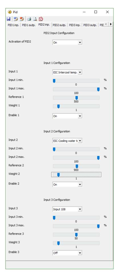
In this example, the ECM (Engine Control Module) measures both the intercooler coolant temperature as well as the jacket cooling water temperature. The generator controller receives these values by an EIC option (Engine Interface Communication).
