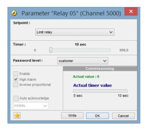
The timer in the image above is an OFF delay, meaning that when the alarm level is OK again, the relay will remain activated until the timer runs out. The timer is only effective when it is configured as "Limit relay". If it is configured to any "Alarm relay", the relay is deactivated instantly when the alarm conditions disappear and it is acknowledged.
