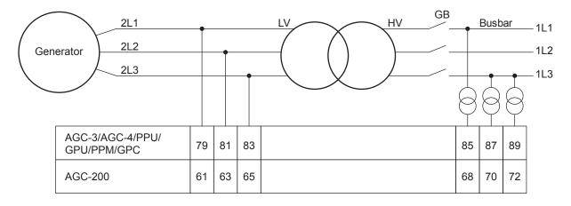
The connection shown in the diagram should always be used when an ML-2 is used for a genset.
