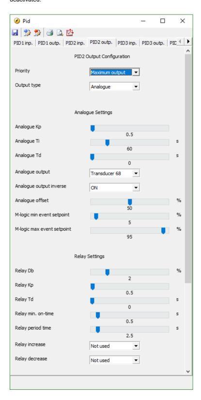
In this application, it is desired to ensure that none of the temperatures permanently exceed their set points. This is achieved by selecting maximum output as priority for the dynamic input selection.
