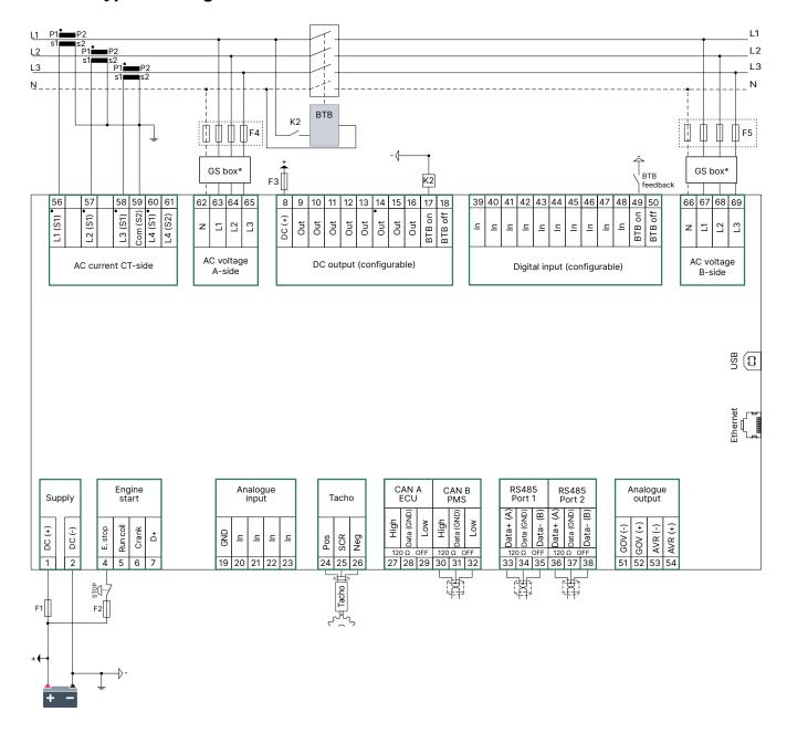
NOTE \* One GS box provides galvanic separation for both sets of voltage measurements.
