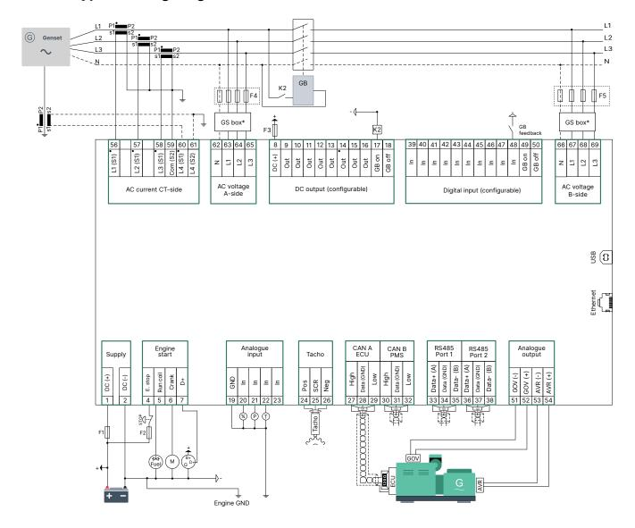
NOTE \* One GS box provides galvanic separation for both sets of voltage measurements.
