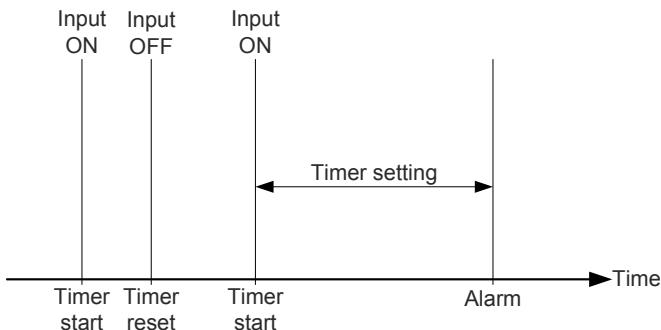
When the delay runs out, the output will be activated.
