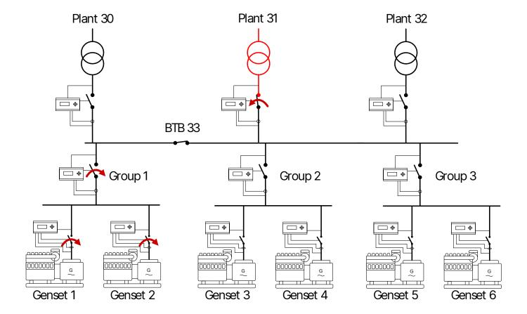
If the plant is set for AMF, or mode shift (7081) is on, when a mains failure appears, the group with the lowest ID gets a start signal. The multi-start setting in the genset controllers determines how many gensets start. The genset(s) then carry the load until the mains is back within normal limits.
