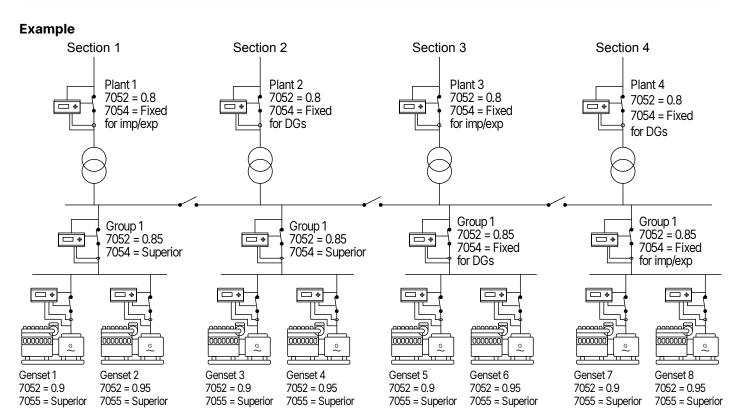
The plant consists of 4 static sections (since the three BTBs are open). The cos phi settings for each controller are shown above.
