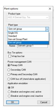
For Plant type, select Genset group. Select the Power management CAN and whether the controllers should be using emulation. After making the selections, select **OK**.
