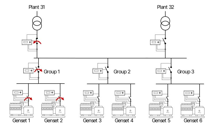
The mains breaker that had previously been closed trips. This can be due to an overload, the breaker's own trip relay, or a digital input configured with the fail class *Trip MB*.
