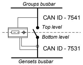
The group controller has two different CAN IDs. In this way, the group controller has two application configurations active at once.
