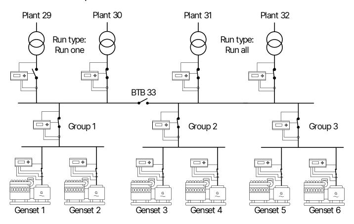
The BTB is open, so the system is divided into 2 static sections.
