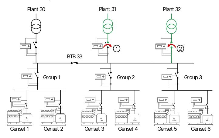
In this application, plant 31 is the *ID to run*, but has had a mains failure. The voltage and frequency are back within normal limits, so the mains feeder can again support the load.
