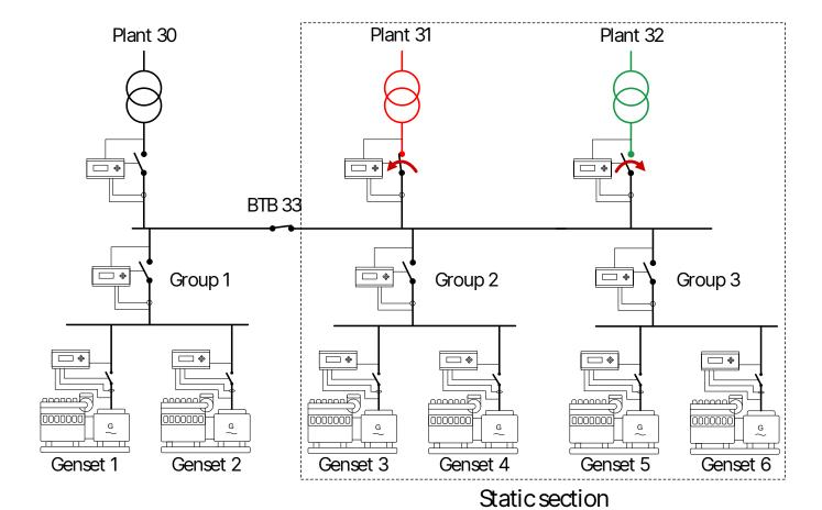
The controllers then check if another mains feeder within its static section is within the voltage and frequency limits, and ready to back up the mains feeder with failure. When auto switch is static section, the controllers can switch to mains feeders within the static section. So if plant 31 has a mains failure, it will switch to plant 32. If this one afterwards has a mains failure, the genset(s) start. The genset group with the first priority receives the start signal.
