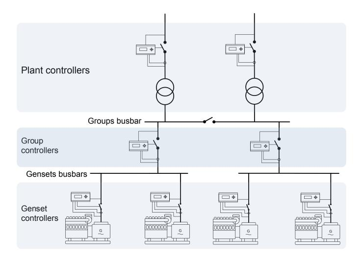
The diagram shows a very simple extended power management application. In this configuration, there are two grid connections. If the plant controllers are removed, the gensets run in island mode. In this way, the controllers can be used in very big island applications.
