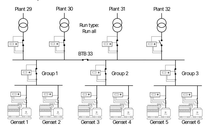
The BTB is closed, so the application consists of one section. The run type is set to run all, and the plant mode is mains power export. Furthermore, the mains feeders are allowed to be parallel.
