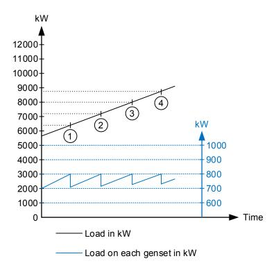
At 5600 kW, the parameters require 8 gensets to supply the load. Gensets 1 to 8 (Group 1) are running. The load increases.
