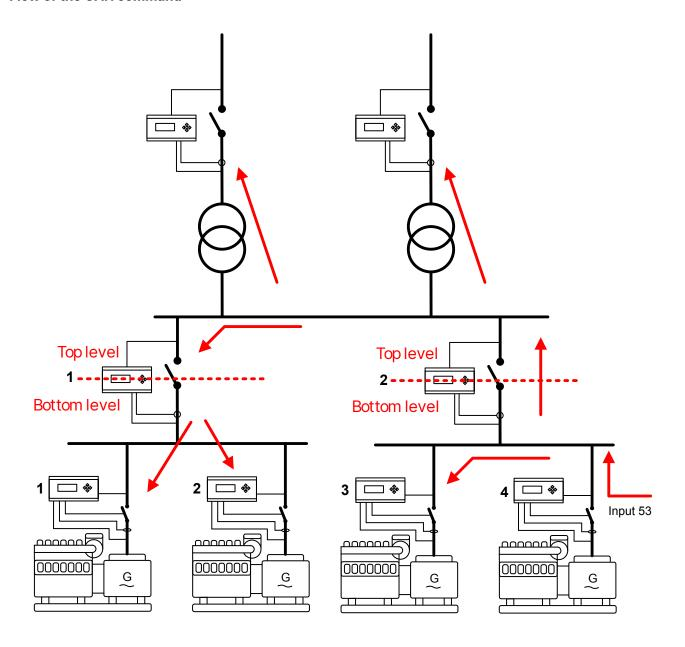
The input is wired to genset 4. When the input is activated, controller 4 activates CAN command 13.
