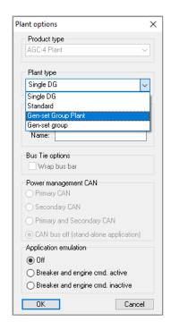
For Plant type, select Gen-set Group Plant. Select the Power management CAN and whether the controllers should be using emulation, then select **OK**.
