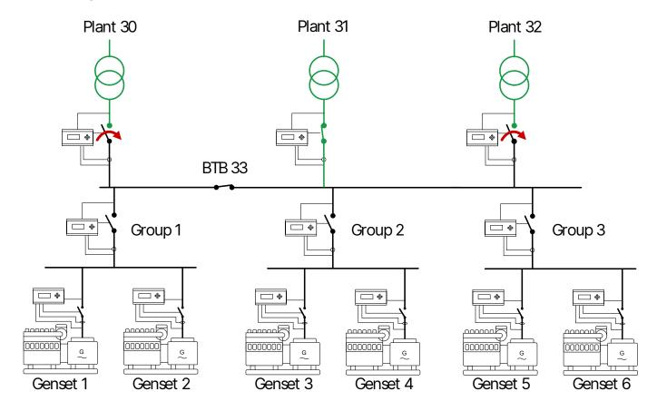
The gensets are not running,. The run type (parameter 8185) is *Run all mains* and therefore all the mains feeders should be parallel when supporting the load. However, the controllers need to know that the mains feeders are allowed to be parallel. When parallel is enabled, the open mains breakers synchronise and close.
