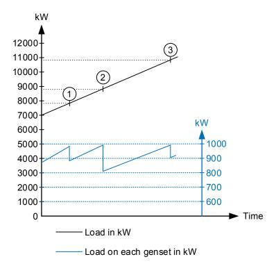
At 7000 kW, the parameters require 8 gensets to supply the load. Gensets 1 to 8 (Group 1) are running. The load increases.
