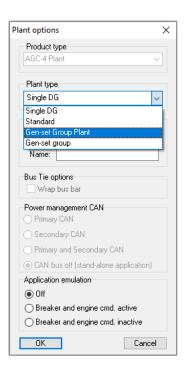
For *Plant type*, select **Gen-set Group Plant**. Select the *Power management CAN* and whether the controllers should be using emulation, then select **OK**.
