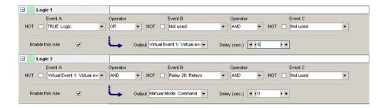
In the above example, the unit will always power up in manual mode. The timer in Logic 1 sets the output for 5 s, and this is used to set manual mode in event 2. When the timer expires, you can freely select any mode since the virtual event 1 turns ON and the Logic 2 says NOT virtual event 1.
