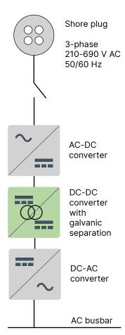
To get the required 3-phase voltage and frequency on the ship busbar, a conventional shore connection may include:
