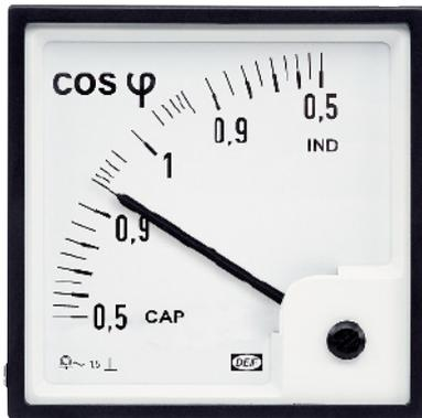
The PFQ power factor meter measures cos phi with a moving coil movement and an electronic transducer. The transducer measures the phase angle between an AC voltage and the corresponding AC current, converting the signal into a proportional DC current which is then fed to the moving coil instrument.
