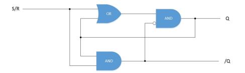
Here the set/reset signal is Virtual Event 1. The output, Q, is connected to an alarm LED.
