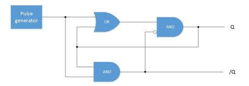
Here the pulse generator is driving the set/reset signal. The set/reset signal is Virtual Event 1. The output, Q, is connected to an alarm LED. Remember the delay time setup for the pulse.
