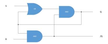
Here the set and reset signals are Virtual Event 1 and Virtual Event 2 respectively. The output, Q, is connected to an alarm LED.
