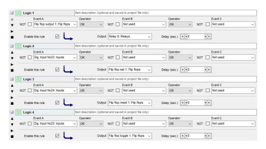
The example shows how flip-flop set 1 could be configured to set relay 8.
