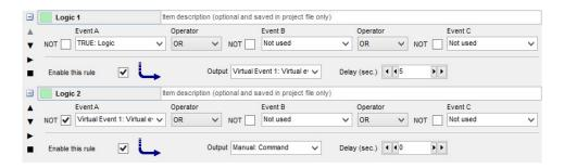
In the above example, the unit will always power up in manual mode. The timer in Logic 1 sets the output for 5 s, and this is used to set manual mode in event 2. When the timer expires, you can freely select any mode since the virtual event 1 turns ON and the Logic 2 says NOT virtual event 1.
