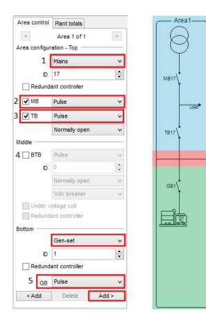
The single-line diagram of the plant is shown on the Application configuration canvas, to the right of the **Area control** window. The single-line diagram has three horizontal sections:
