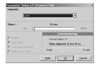
The timer adjusted in this dialog box is the off delay which is shown in the above drawings.
