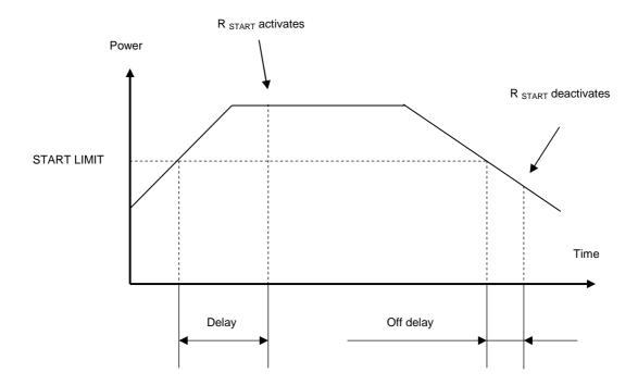
The load dependent start relay reacts based on the power measurement of the GPU only. It is not dependent on a running signal from the gen-set or the CB position (these signals are not monitored by the GPU).
