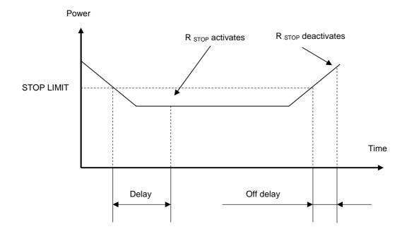
The load dependent stop relay reacts based on the power measurement of the GPU only. It is not dependent on a running signal from the gen-set or the CB position (these signals are not monitored by the GPU).
