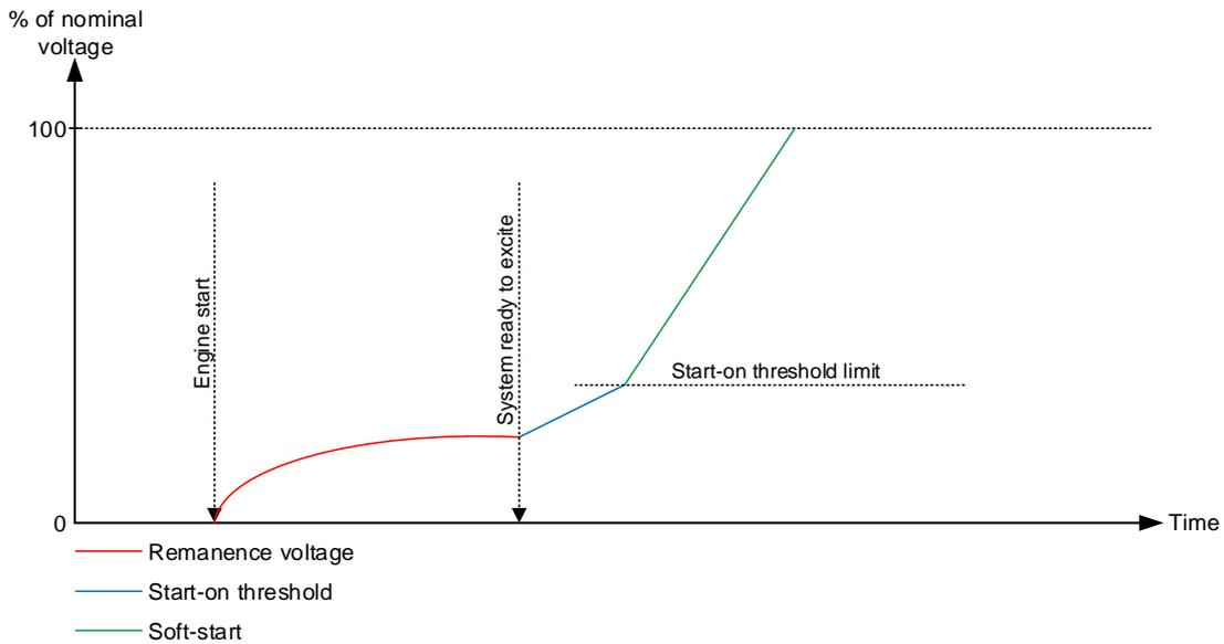
The soft-start timer in CBE is not the same as the soft-start timer in normal start, but the start-on threshold parameters are the same as in the normal start. Having different settings for the soft-start gives the possibility to have for example a more aggressive excitation ramp for CBE sequences. The timer for the soft-start in CBE is located in parameter 2262. Note that this timer is different from the one in normal start.
