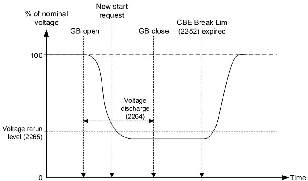
In the diagram above, the excitation is shut off as soon as the breaker is opened. Shortly after the breaker is opened, a new start request appears. The Multi-line 2 unit will wait with the closing of the GB until the “voltage discharge timer” has expired.
