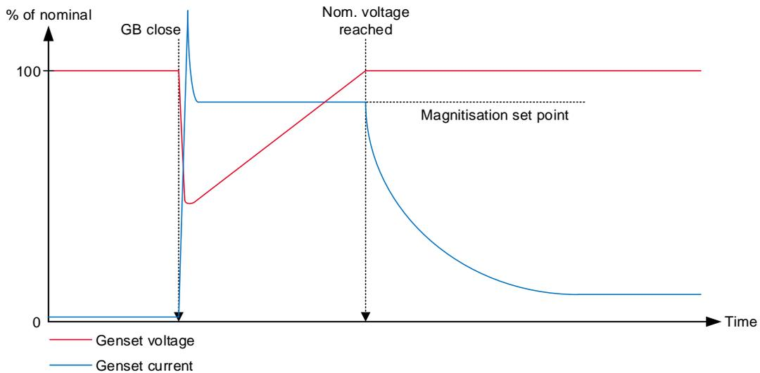
The first dotted line shows when the generator breaker closes. The second dotted line shows when the transformer magnetisation function will be deactivated (5 % below the current limitation set point set at parameter 7793).
