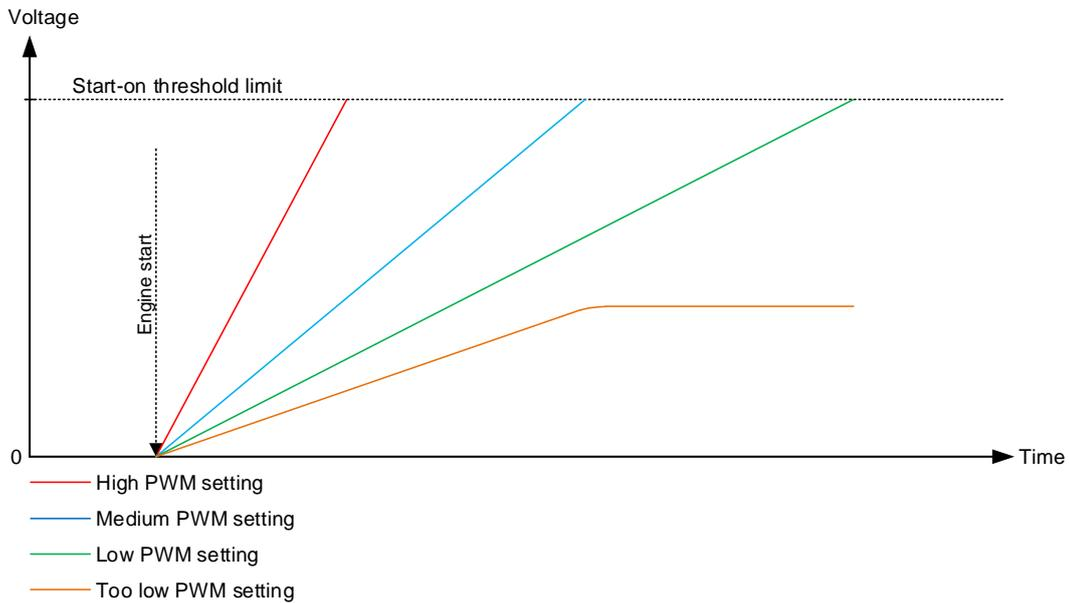
When the upper limit for the start-on threshold is changed, the start point for the soft-start is also changed. The upper limit for start-on threshold is always the start point for soft-start.
