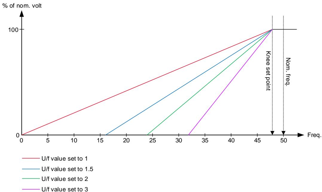
The knee set point determines when the U/f law becomes active. When the frequency goes below the knee set point, the U/f law defines a temporary voltage set point for the DVC 310.
