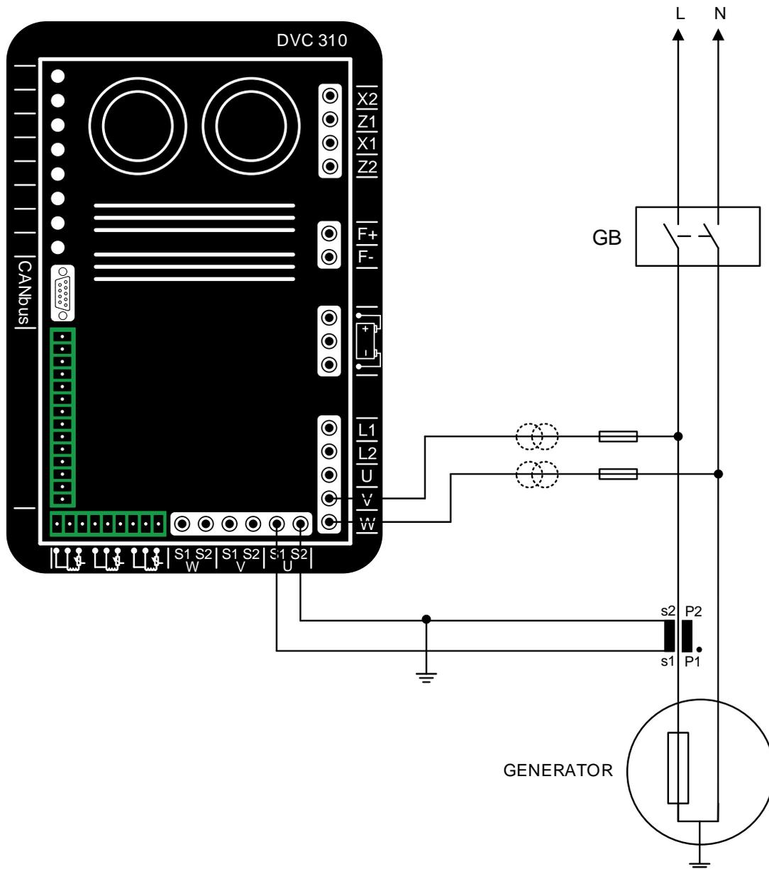
For the DVC 310 to measure correctly, the current transformer will need a phase correction, which is set in the EasyReg software. In the EasyReg software, this is configured in the "Generator setting - Options" window.
