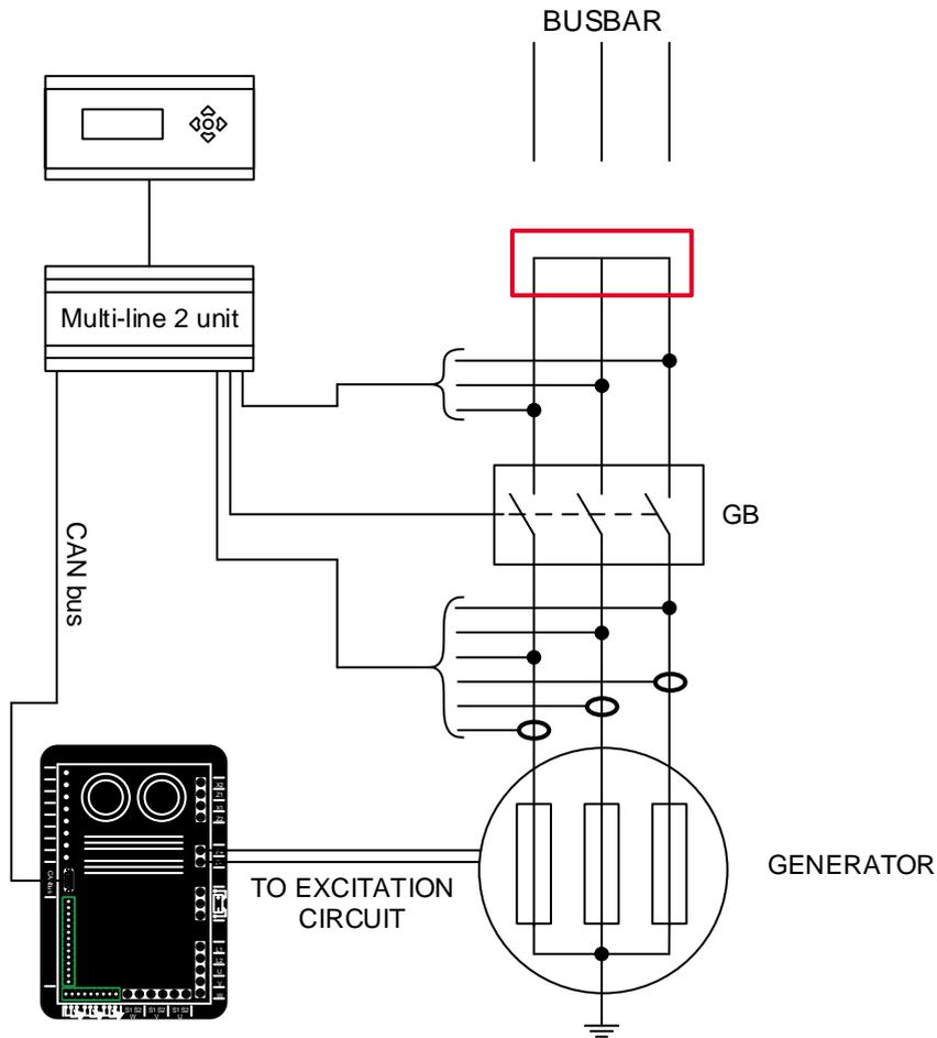
2. Choose Dry alternator mode at parameter 6071. Start the genset in semi-auto mode and close the GB. When the windings are dried out, open the GB and stop the genset.
