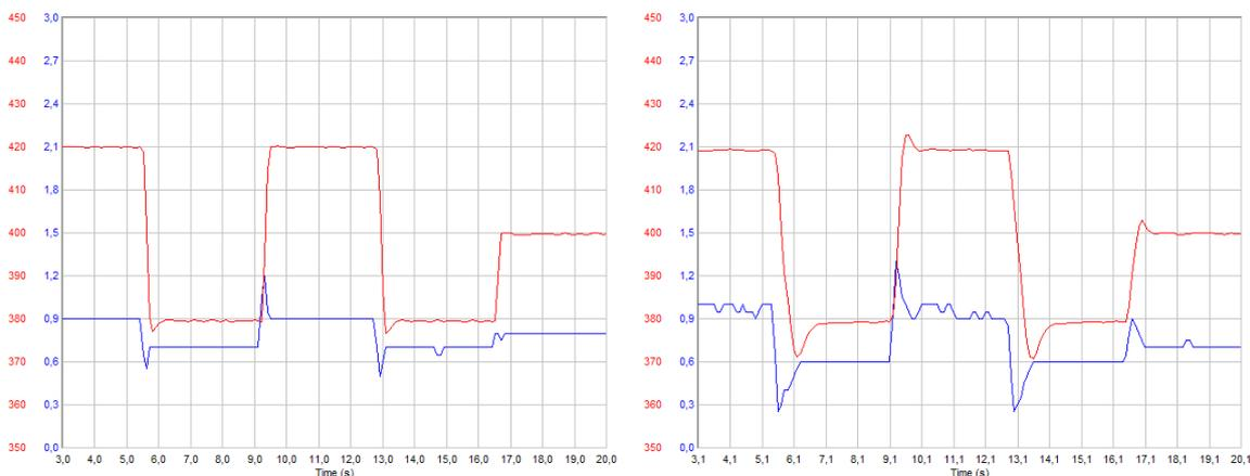
When the regulation has been tuned sufficiently, the "soft-start" ramp can be tuned down until the user finds the start up ramp fast enough.
