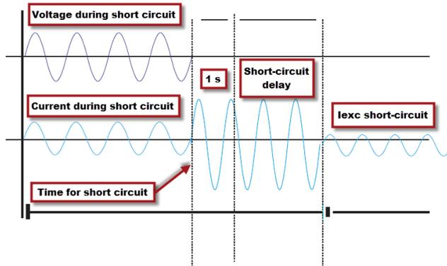
The short circuit protection is activated at parameter 7825:
