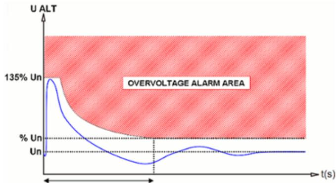
The over-voltage protection in the DVC 310 is enabled in parameter 7823:
