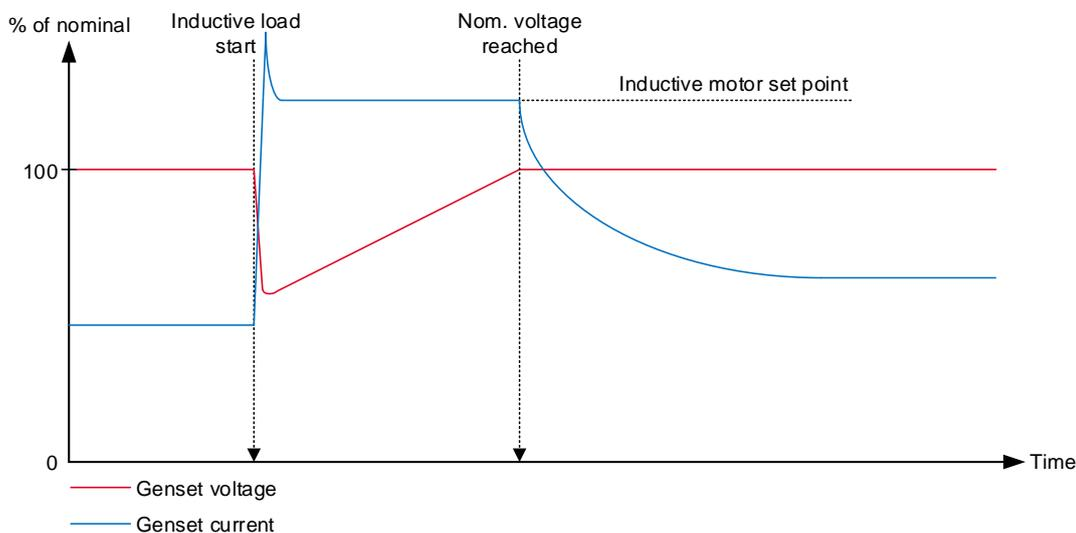
When the inductive load is turned on, the current will rise. The inductive motor function will limit the current to the predefined level set in parameter 7794. The DVC 310 will change to have the current as set point and let the voltage drop. When the voltage reaches the nominal value again, the DVC 310 will change to regulate with the voltage as set point again.
