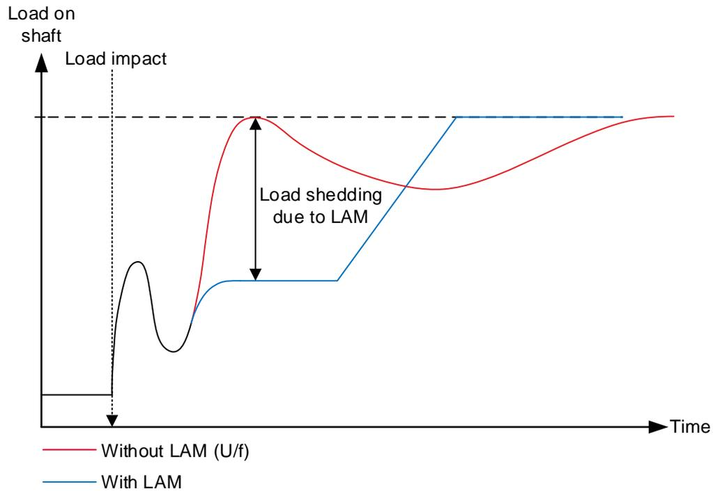
The graph above shows a comparison of the load on the shaft of the engine, with the LAM function enabled and disabled. When the LAM function drops the voltage, the torque on the shaft is lightened, which makes it possible for the engine to rise faster in RPM after a load impact. This also gives the possibility to steadily reach nominal values faster after the load impact, since the LAM function will increase system stability.
