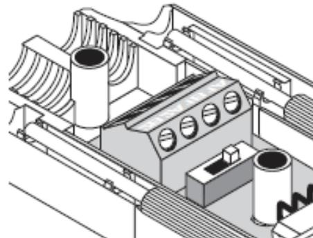
Check the setting of the terminal resistor when the wiring is done. It can be set to ON or OFF on the switch next to the terminals in the included CAN connector.
