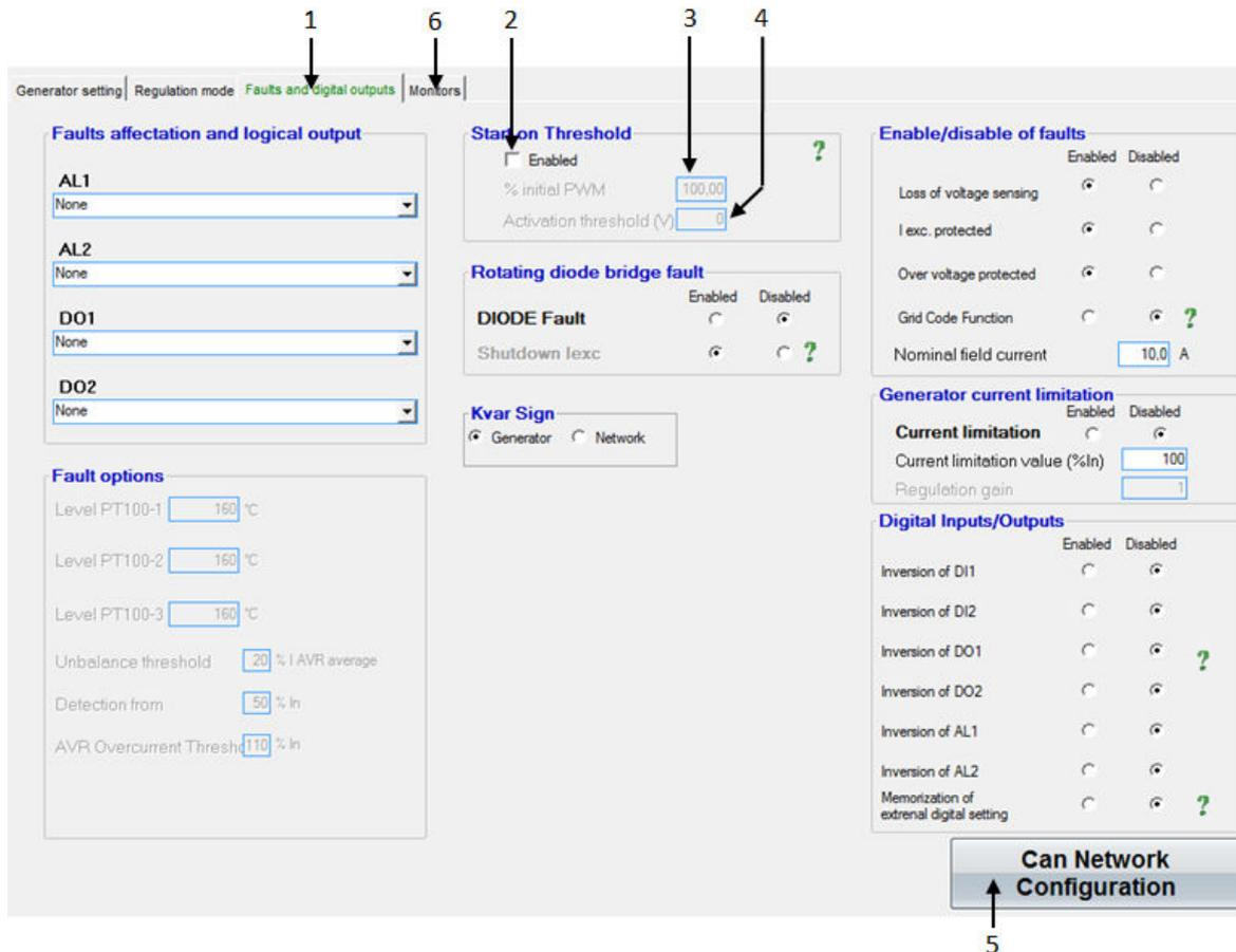
1. Here the "Fault and digital inputs" tab can be pushed, and then the window should look like above.
