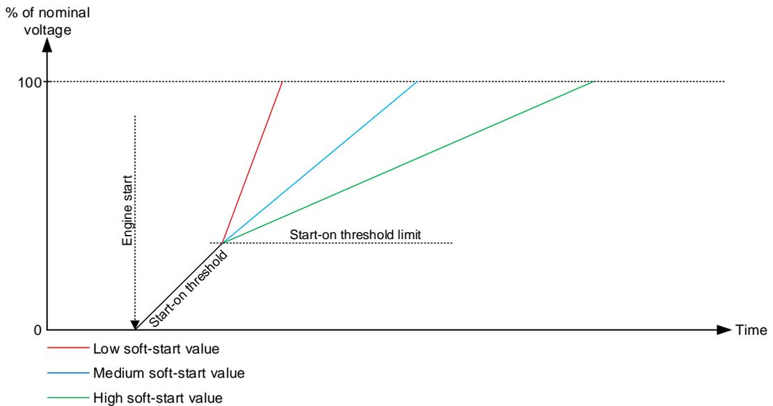
Since the soft-start timer represents how much time it should take to ramp up the voltage from 0 V to nominal, the full timer will not be used if the start-on threshold function is also used. If the wanted duration of the soft-start is known, the timer to set in the parameter can be calculated instead:
