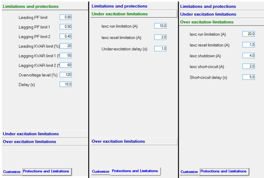
The three windows contain different settings. Some of them are used when the DVC 310 is interfaced with a Multi-line 2 unit. In the first window, only over-voltage and delay are used. None of the settings in the second window are used. In the third window, all settings are used. In the settings that are not used, a proper value must be entered. Refer to the chapter "Protections" for a description of all protections.
