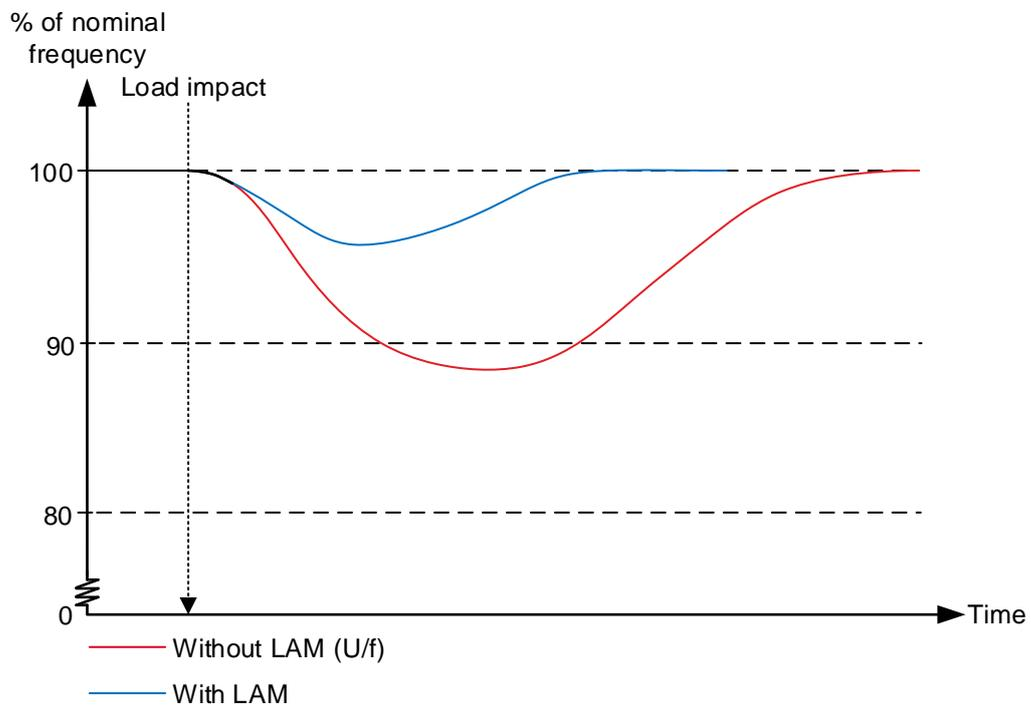
The graph above shows that with the LAM function, the frequency will rise and stabilise faster after a big load impact. This is because the LAM function will drop the voltage and by this lower the torque on the engine.
