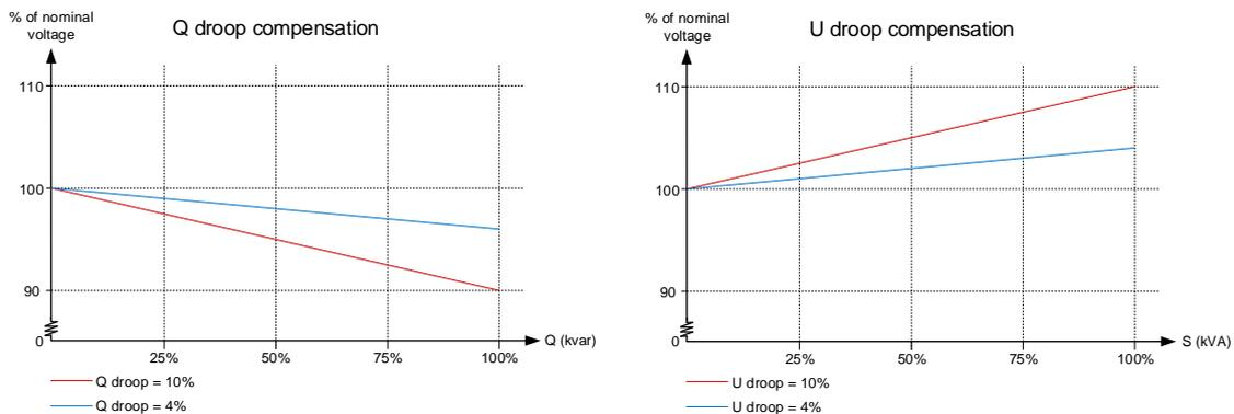
The droop compensation decides how much the voltage is allowed to droop if the regulation is turned off in the Multi-line 2 unit. The regulation can be turned off by setting the Multi-line 2 unit into MANUAL. The regulation can also be off if the CAN bus cables should break. With the droop, it is possible to give the DVC 310 a set point for the voltage if an error in the CAN bus lines should occur. This makes it possible for the genset to share the reactive load when no interfacing is available.
