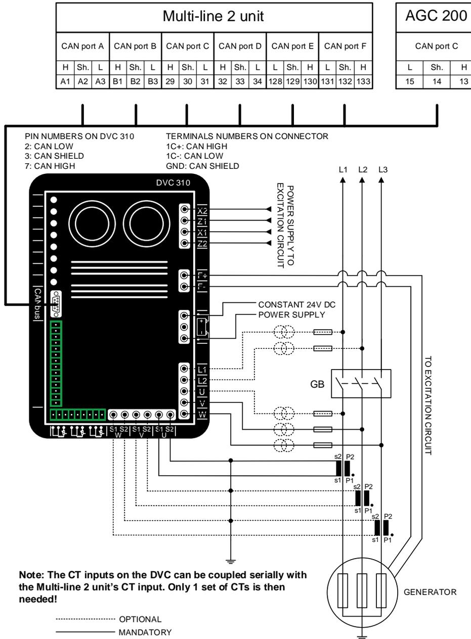
**i** The CT inputs on the DVC 310 can be coupled serially with the Multi-line 2 unit's CT input. In that case, only one set of CTs is needed.
