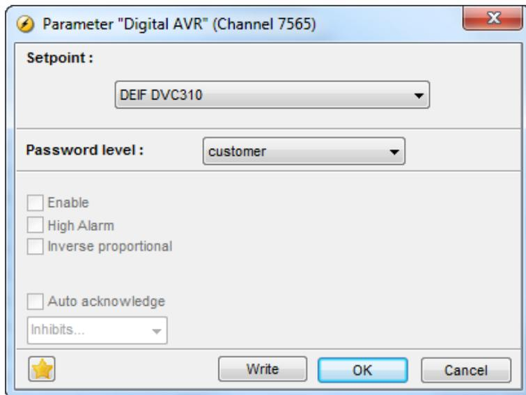
At last, the engine interface must be set; this is done at parameter 7561. It must be set even though relay or analogue regulation is used for governor control, and it must be set to anything else than OFF.
