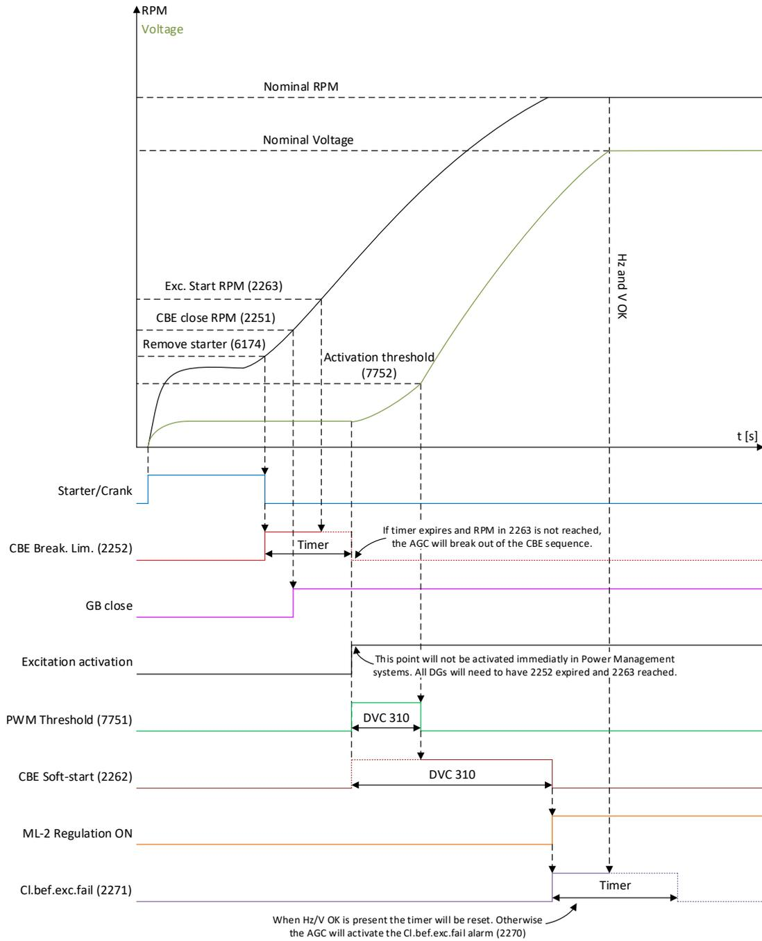
Please note, that the soft-start ramp time is started, when the excitation is started. The soft-start timer should be considered as an angle of slope, instead of a specific time.
