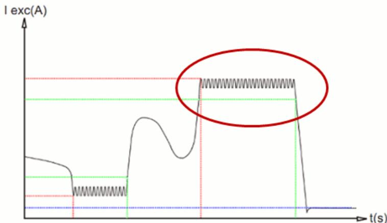
If the genset is supporting a very inductive load, the magnetic flux density in the rotor can be very high, which can cause end-turn burning. This protection contains three parameters, which can all be found in the Easy-Reg software.
