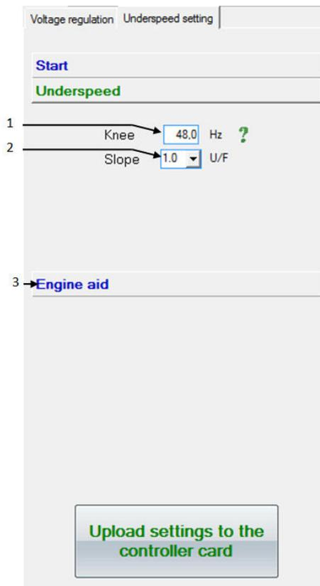
1. This setting determines the upper limit for the U/f slope. If there is a load impact on the genset, and the frequency reaches this set point, the DVC 310 starts slope on the voltage. The knee function is described in the section "U/f (knee function)".
