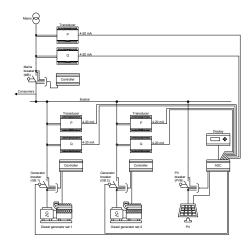
The maximum capability of the stand-alone applications is 16 gensets, one mains and one PV plant.
