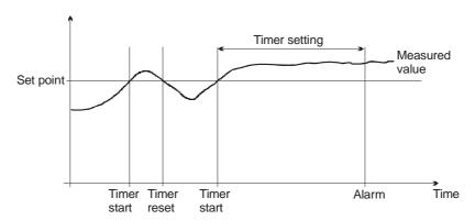
When the timer runs out, the output is activated. The total delay will be the delay setting + the reaction time.
