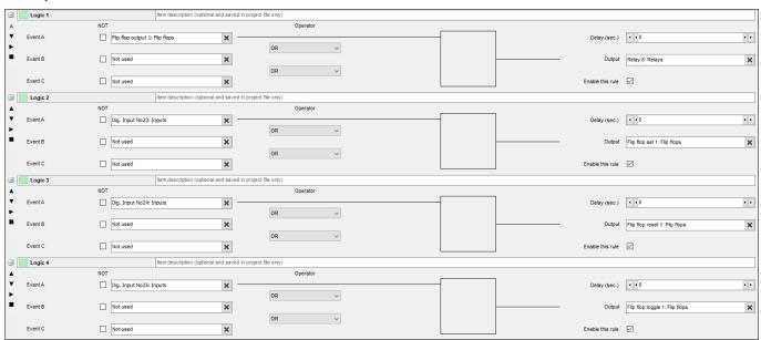
The example shows how flip flop set 1 could be configured to set relay 8:
