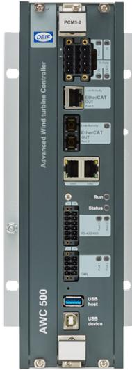
DEIF's PCM5-2 Power and Control module, for the AWC 500 series offers processing power and gigabit network connectivity at data server level. Without compromising on its capability to cope with the toughest climate demanding environments, the PCM5-2 is a rugged and reliable PLC well suited for distributed and remote energy generation for example wind turbines.
