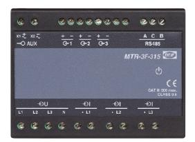
The size of a portable hard drive, the MTR-3 transducers are slight in size but each one offers equal performance of up to four standard transducers, measuring and calculating AC voltage, AC current, active/reactive/apparent power, power factor, frequency, kWh, kvar, THD, dynamic and maximum demands.
