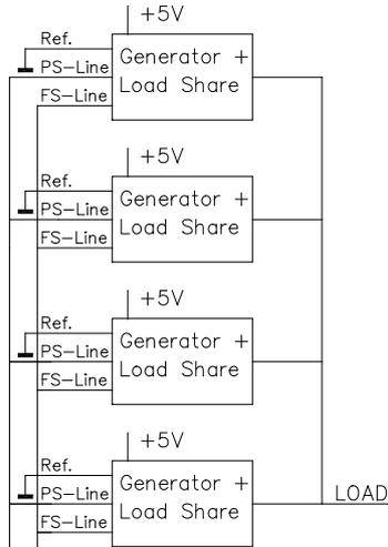
Fixed load to busbar - No frequency control
