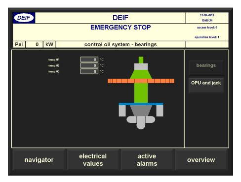
There are up to 20 configurable temperature indicators available. For each, the text, input and alarms can be configured freely. Similar screens are available for Francis and Pelton turbines.
